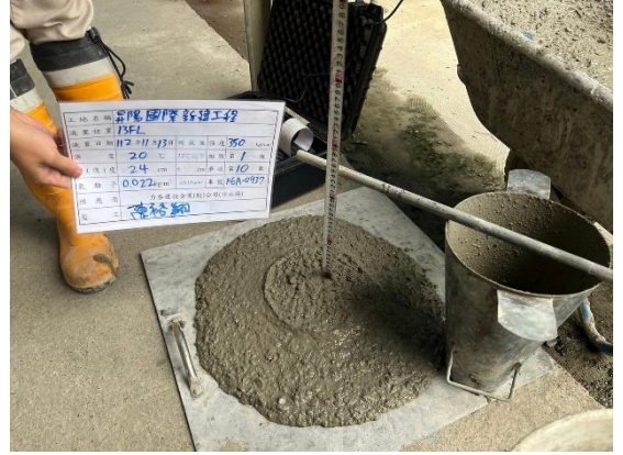
混凝土坍度試驗
